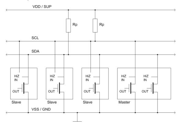
Pull-up resistors are needed at SDA and SCL. 1..10kOhm are recommended. In order to optimise the data rate or low power consumption, other resistance values are possible.
