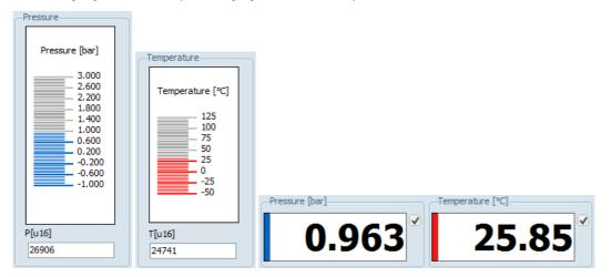
The scaling of a D-Line transmitter is always in [bar] and [°C]. There are two ways to convert the figures to other units.
